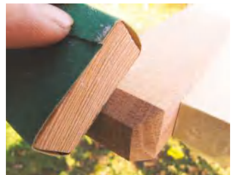
STEP 12. If necessary, you can tidy up your routed chamfers with a few strokes from a sanding block
